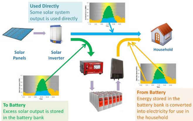
**Electricity Flows for a solar system with battery storage**
