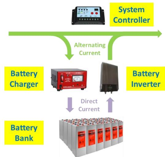
Components of a battery storage system
