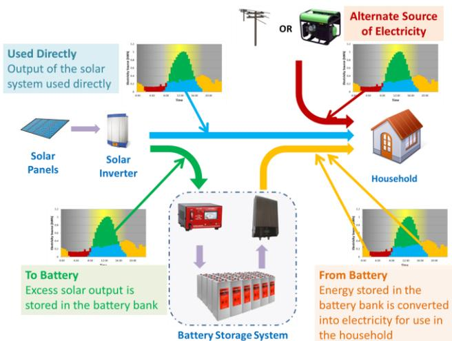
Showing an alternate source of electricity able to supply power when the battery bank is empty
