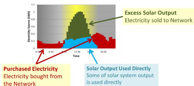
Electricity flows with a network connected solar system
