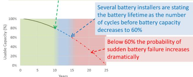
Typical usable battery capacity for quality storage batteries
