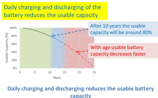
Battery degradation is not linear. As shown in the figure the rate increases with age. This explains why we notice the limited runtime of a 2 year old mobile phone. Once the usable capacity falls below 80% battery degradation is accelerating and the daily runtime becomes noticeably shorter each week.
