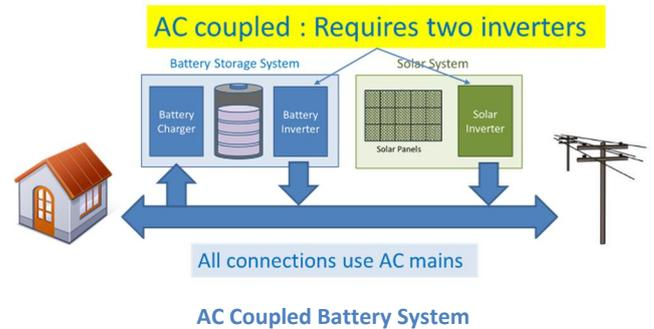
As noted in the above figure AC coupling is requires two inverters, one for the solar system and one for the battery system. Both inverters basically do the same job suggesting it is possible to remove one.
