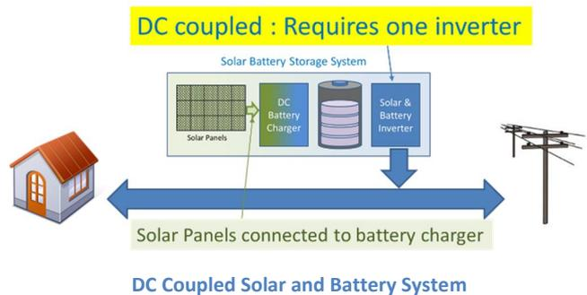
The solar inverter accounts for 10 to 15% of the total cost of the solar system. Choosing to install a DC coupled solar/battery storage system potentially reduces the price by nearly \$1000.
