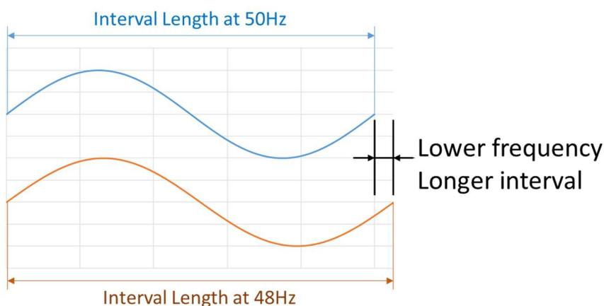
The problem is slower mains frequencies coincide with the Peak Time of Use period. Summating interval data to calculate energy use during the Peak periods is likely to include a systematic measurement bias, in favour of the utility.
